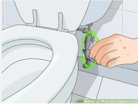
**2** Turn the valve clockwise until it can't turn anymore. Turning the valve clockwise as far as it can go will turn off the water supply to the toilet. The valve should not be difficult to turn, so don't try to force it if you can't easily turn it.<sup>[2]</sup>
