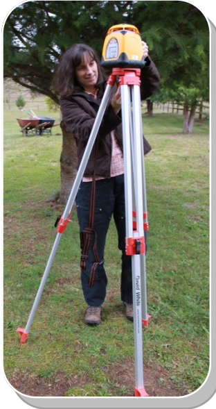
Teresa Brooks, former OC Intern, sets up an electronic level at a new rain garden site.
